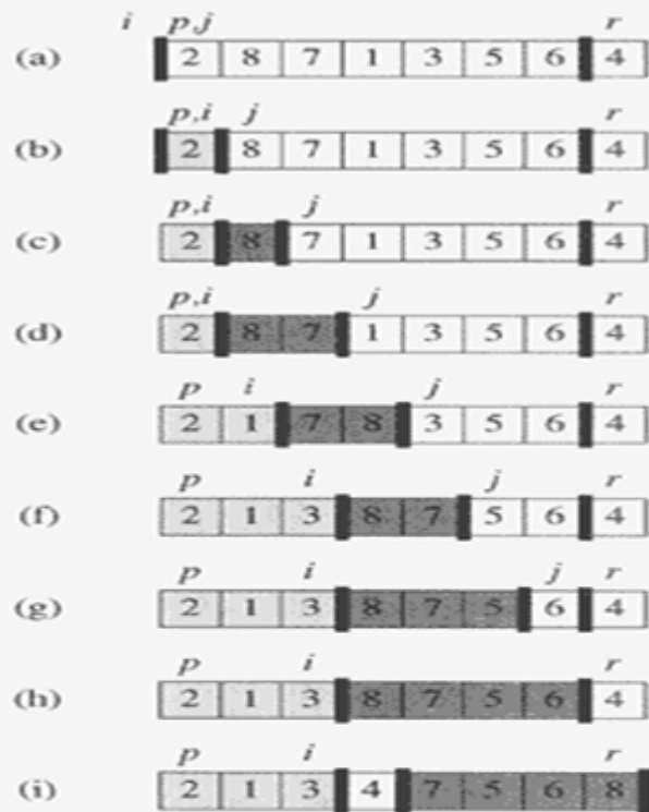
Figure 7.1 The operation of PARTITION on a sample array. Lightly shaded array elements are all in the first partition with values no greater than x . Heavily shaded elements are in the second partition with values greater than x . The unshaded elements have not yet been put in one of the first two partitions, and the final white element is the pivot. (a) The initial array and variable settings. None of the elements have been placed in either of the first two partitions. (b) The value 2 is “swapped with itself” and put in the partition of smaller values. (c)–(d) The values 8 and 7 are added to the partition of larger values. (e) The values 1 and 8 are swapped, and the smaller partition grows. (f) The values 3 and 8 are swapped, and the larger partition grows. (g)–(h) The larger partition grows to include 5 and 6 and the loop terminates. (i) In lines 7–8, the pivot element is swapped so that it lies between the two partitions.
